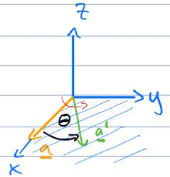
$$\Rightarrow \underline{a}' = \underline{G}(1,2,\theta) \cdot \underline{a} = \begin{bmatrix} c & -s & 0 \\ s & c & 0 \\ 0 & 0 & 1 \end{bmatrix} \cdot \begin{bmatrix} 1 \\ 0 \\ 0 \end{bmatrix} = \underline{\underline{\begin{bmatrix} \cos\theta \\ \sin\theta \\ 0 \end{bmatrix}}}$$
