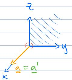
$$\Rightarrow \underline{a}' = \underline{G}(2,3,\theta) \cdot \underline{a} = \begin{bmatrix} 1 & 0 & 0 \\ 0 & c & -s \\ 0 & s & c \end{bmatrix} \cdot \begin{bmatrix} 1 \\ 0 \\ 0 \end{bmatrix} = \underline{\underline{\begin{bmatrix} 1 \\ 0 \\ 0 \end{bmatrix}}}$$
