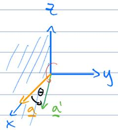
$$\Rightarrow \underline{a}' = \underline{G}(1,3,\theta) \cdot \underline{a} = \begin{bmatrix} c & 0 & s \\ 0 & 1 & 0 \\ -s & 0 & c \end{bmatrix} \cdot \begin{bmatrix} 1 \\ 0 \\ 0 \end{bmatrix} = \underline{\underline{\begin{bmatrix} \cos\theta \\ 0 \\ -\sin\theta \end{bmatrix}}}$$
